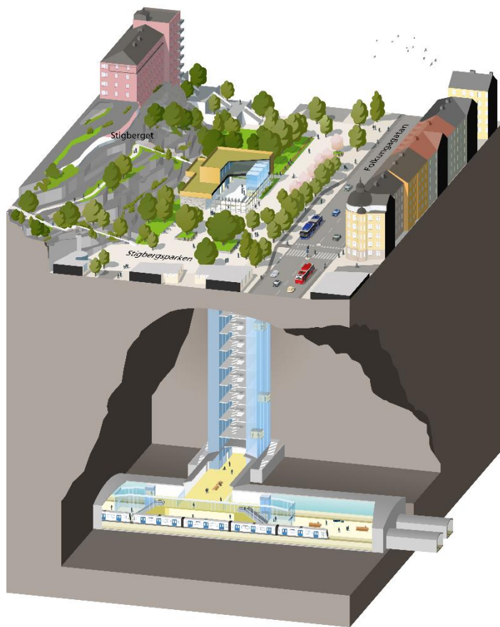
Cross-section of the future Sofia metro station with the Stigberg Park above (image: Stockholm Region / Sweco)
