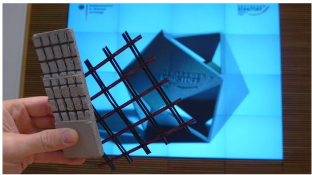
Carbon concrete composite, a composite of carbon fibres and high-performance concrete, opens new possibilities in construction and in architecture. Implenia is working within the award-winning C<sup>3</sup> Consortium on improving the new composite, developing basic design principles and identifying potential applications. (Picture: C<sup>3</sup>- Carbon Concrete Composite e.V.)
