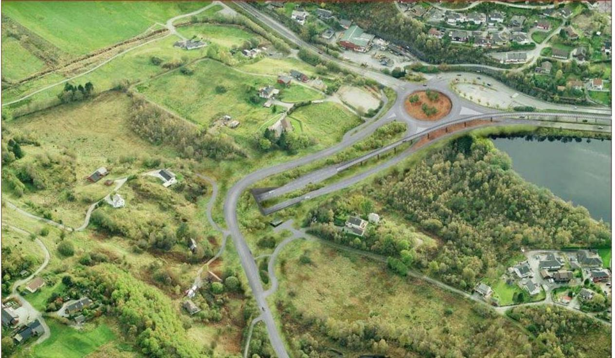
The contract for the upgrade of a section of the four-lane E39 motorway between Vagsbotn and Hylkje on Norway's west coast comprises – in addition to the road construction works – two 600-metre tunnels, four portals, a concrete viaduct, and three smaller bridges, as well as separate lanes for pedestrians and cyclists.
