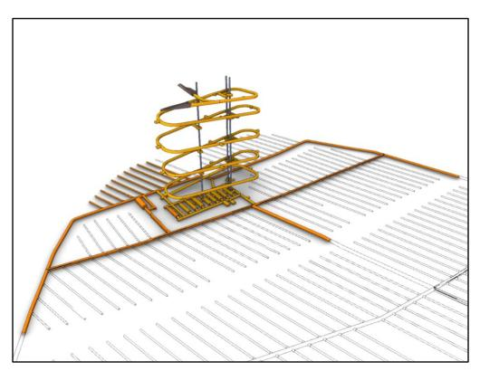
The scope of the contract with Implenia includes the planning, design and construction of an access tunnel to the first storage level, three vertical shafts for ventilation and an elevator, a central area as well as main and transport tunnels (image: ©SKB).
