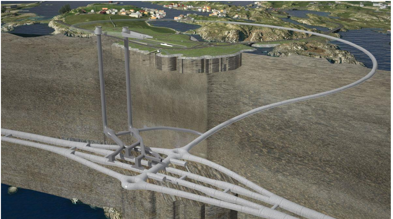
Project E02 Kvitsøy, E39 Rogfast: A large and complex tunnelling system at approximately 230 m below sea surface (image: © Norconsult/Norwegian Public Roads Administration).
